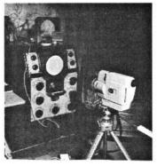
Fig. 10. The Cossor 1039 MKIII doublebeam scope used for the examples Fig. 8 and 9. This model employed valves and the Y amplifier inputs catered for d.c. as well as a.c. voltages. (The cine camera was used to make a demonstration film of oscilloscope applications).
